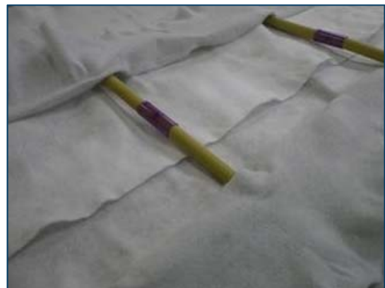
Figures 6: Transverse connections with couplers
