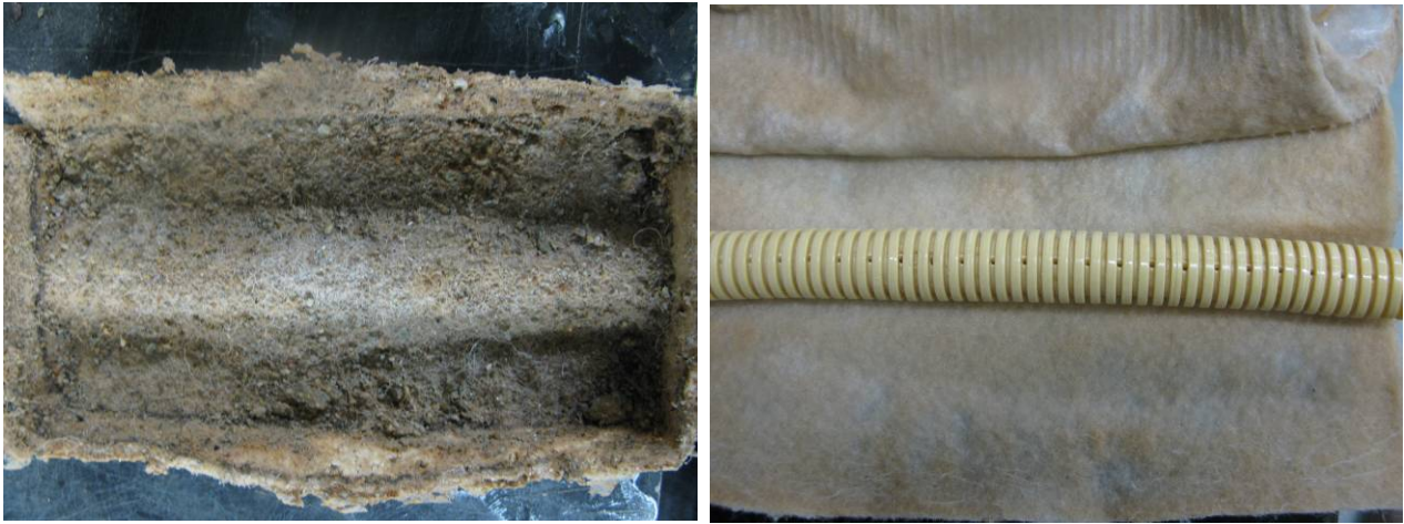
Figure 4: External and Internal View of the Geocomposite after Three Months of Percolation of Sulfuric Acid
