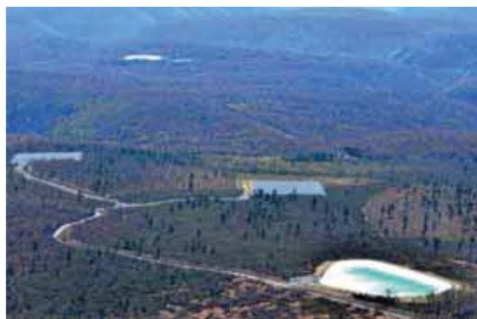
and cover soil stability should always be evaluated and may affect the selection of the liner. Common geomembrane liner materials are 40- or 60-mil textured LLDPE or HDPE geomembranes.
