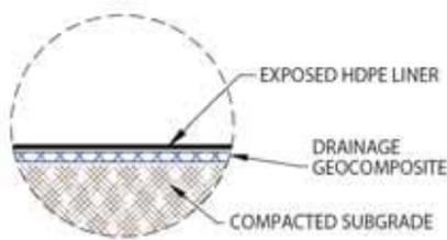
FIGURE 2 Typical liner system cross section.
